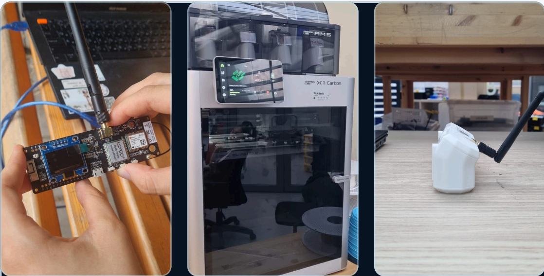
Prototype path: electronics integration → additive manufacturing → enclosed field-ready form.
