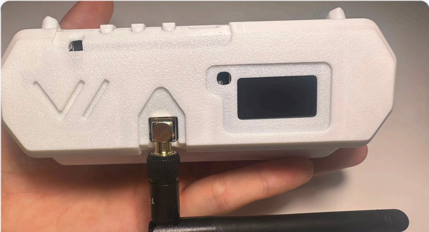
Final handheld prototype — OLED, antenna and enclosure geometry
