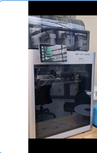
Bambu X1-Carbon and printed enclosure evidence
