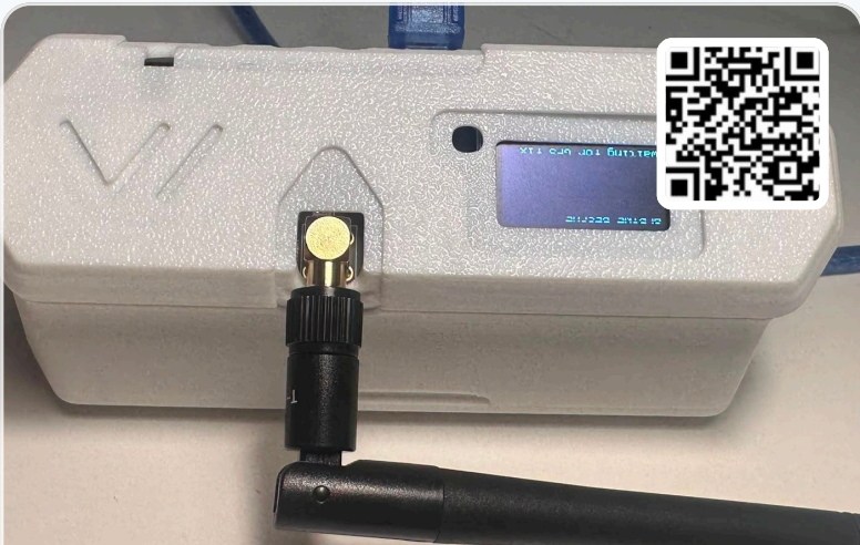
Final beacon enclosure with Device ID / QR label zone
