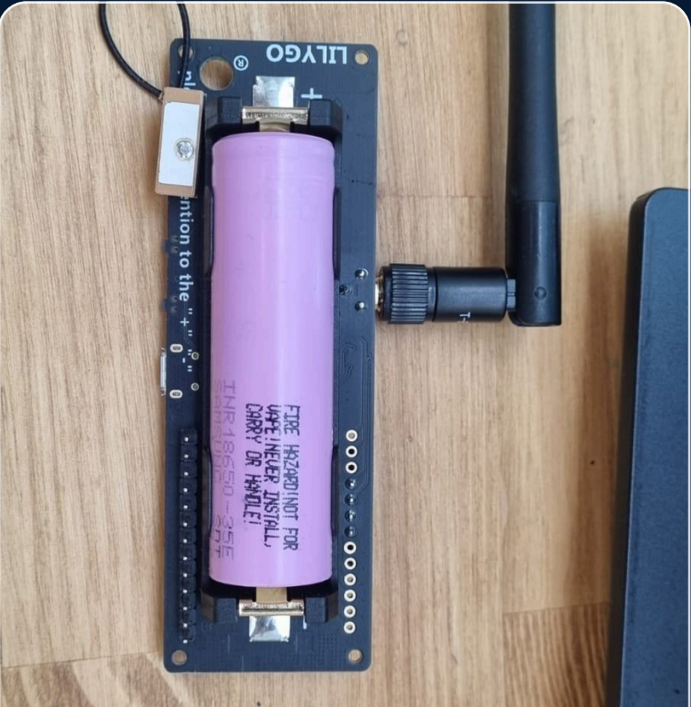
18650 cell installed on the T-Beam power side
